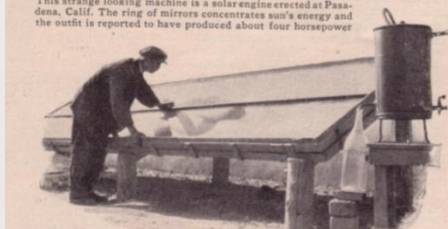
This strange looking machine is a solar engine erected at Pasadena, Calif. The ring of mirrors concentrates sun's energy and the outfit is reported to have produced about four horsepower
